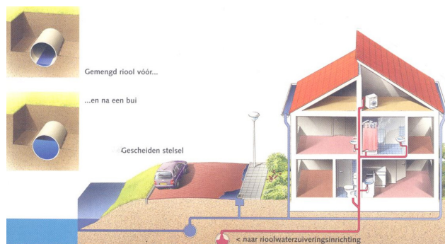
Gescheiden riolering – bron Rioned
